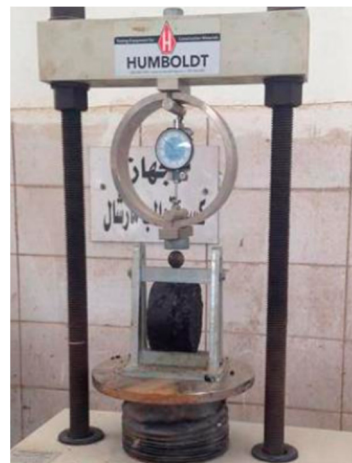
Figure 7. Instrument for indirect tensile test.
