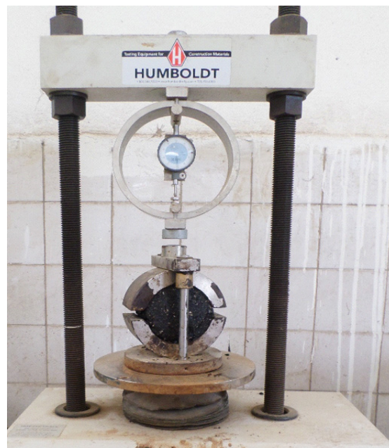
Figure 4. Marshall test (HUMBOLDT).
